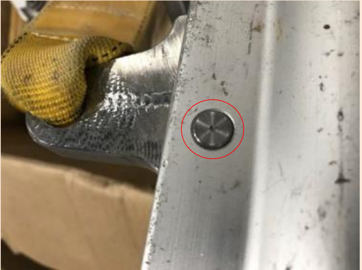
IMAGE 2: Additional example of dimple markings on Cougar Trolley 3.0 knurled
