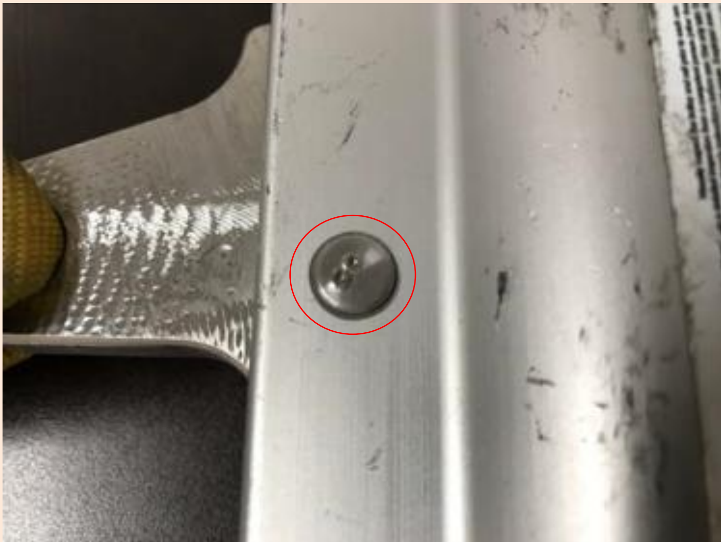
IMAGE 1: Example of dimple markings on Cougar Trolley 3.0 knurled pin
